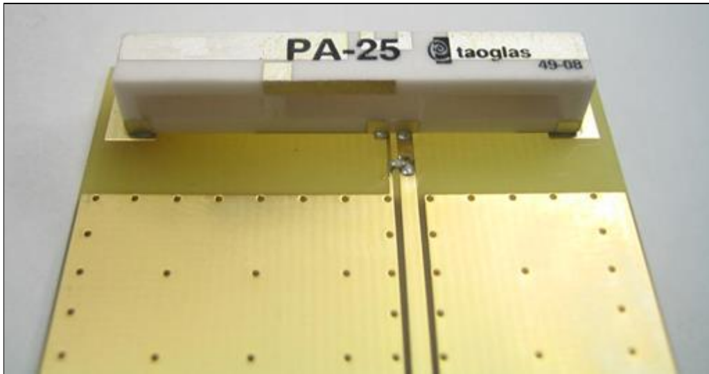
Figure 18. Antenna location on EVB (front view)..
