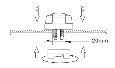
Recommended Torque setting for mounting is 24.5N·m Maximum Torque setting for mounting is 29.4N·m.
