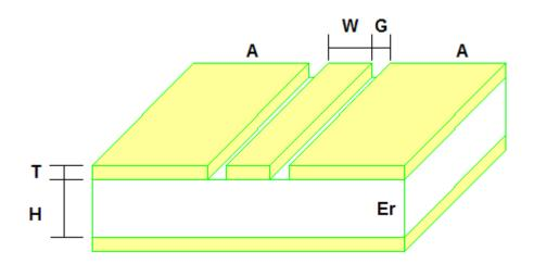
Figure 2. Representation of Co-Planar Waveguide (CPW).
