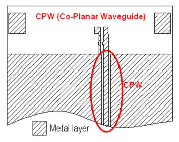
Figure 3. Co-Planar Waveguide (CPW).
