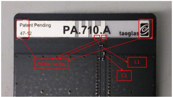
Figure 6. Layout for the Matching circuit.
