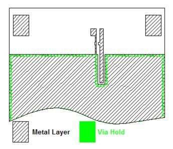
Figure 4. Via holes fence.
