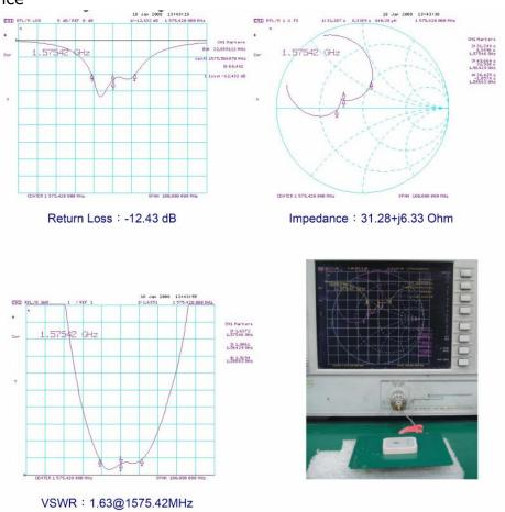
The antenna is physically tuned a number of ways, the shape of the top silver electrode can be changed, or the feed-point can be moved.
