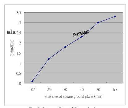
Fig. 2 Gain vs Size of Ground-plane
