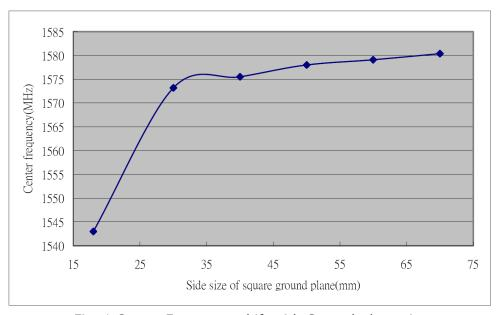
Fig. 1 Centre Frequency shift with Ground-plane size
