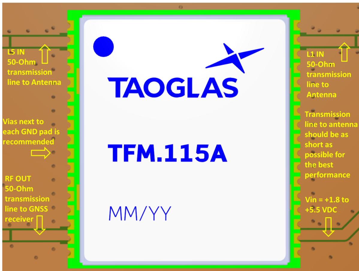
TFM.115A module mounted on a PCB, showing transmission lines and integration notes.
