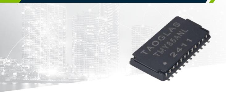
Featuring a compatible footprint with industry LAN transformers, and designed to work in demanding industrial environmental conditions, the Taoglas TMY85ANL is a 1G Base-T Single Port of 24pin with 3 Wire and Transformer designed for PoE applications.
