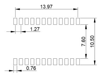
Suggested pad layout Dimensions are in millimeters with the following tolerances: X.XX =  $\pm 0.10$
