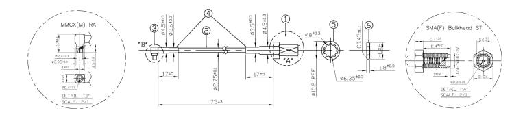
CAB.01044 RG-174 75mm CAB.01046 RG-174 300mm
