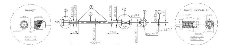
CAB.01040 RG-174 300mm CAB.01041 RG-174 250mm CAB.01042 RG-174 200mm CAB.01043 RG-174 150mm CAB.0102 RG-174 100mm
