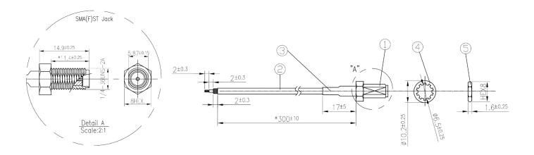
CAB.01030 RG-174 300mm CAB.01031 RG-174 250mm CAB.01032 RG-174 200mm CAB.0125 RG-174 150mm
