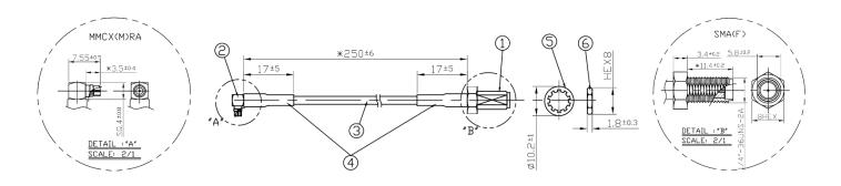
CAB.01045 RG-174 250mm CAB.0171 RG-174 150mm
